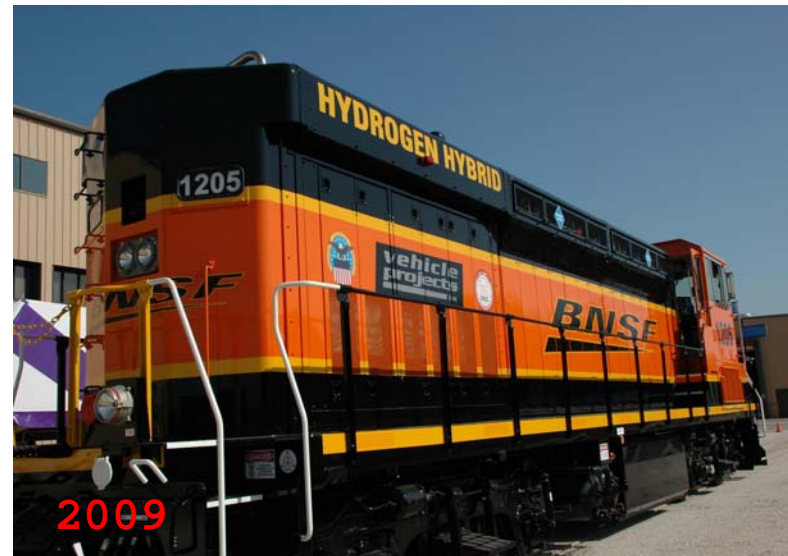
127 t, 1.6 MW (max) fuelcell-hybrid shunting locomotive
